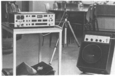
Fig.2. The Sound Source Type 4224 fitted with its diffuser. Here used in conjunction with the Building Acoustics Analyzer Type 4418 to measure reverberation time in a cafeteria
